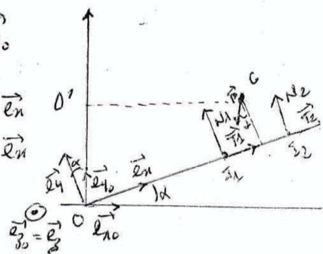
$$-\frac{Mv^2}{\rho} \cos \alpha = -Mg \sin \alpha + T_{1x} + T_{2x} \quad (1) \quad (\text{eq. 1})$$
